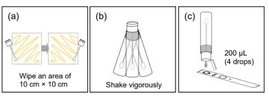
Fig. 2. Test steps for swab test sample
